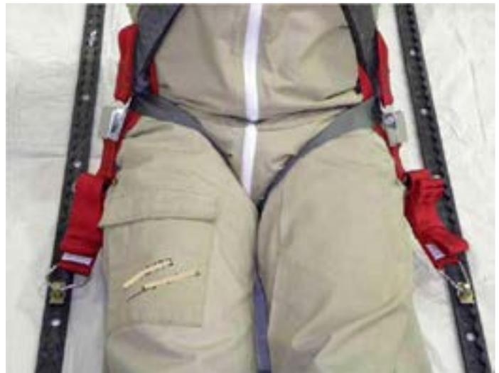
Figure 6. Latch Tether Loop Around Parachute Harness
