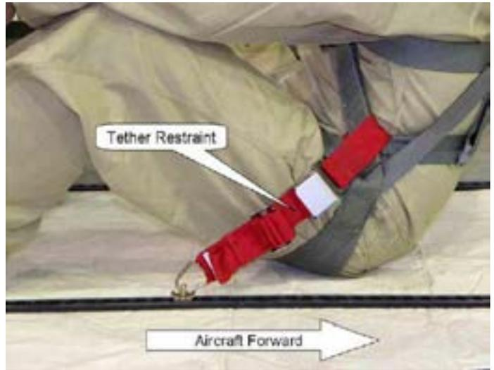
Figure 5. Pass Tether Loop Under Main Lift Web
